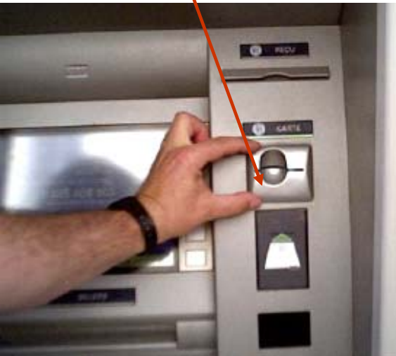
Figure 1B: A card reader overlay is installed on the ABM
