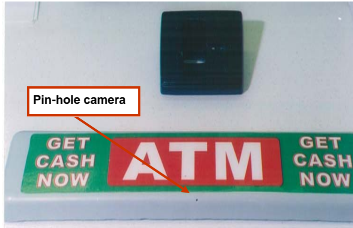
Figure 3: A false topper is attached to ABM to conceal a pin-hole camera
